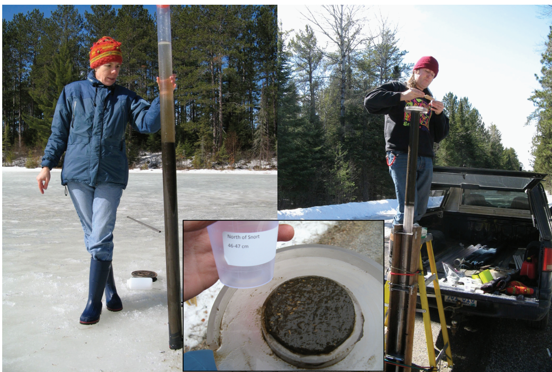
Lake sediment cores collected from the eastern and western regions of the Mesabi Iron Range offer insights into historic production of mineral dust. Example of lake sediment core sampling at “North-of-Snort” Lake by scientist Lisa Allinger (left) and Dr. Euan Reavie (right).
